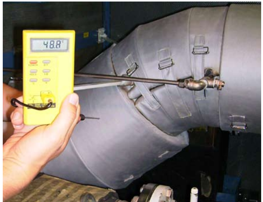
... to below 50°C (122°F) with the thinner aerogel solution.
