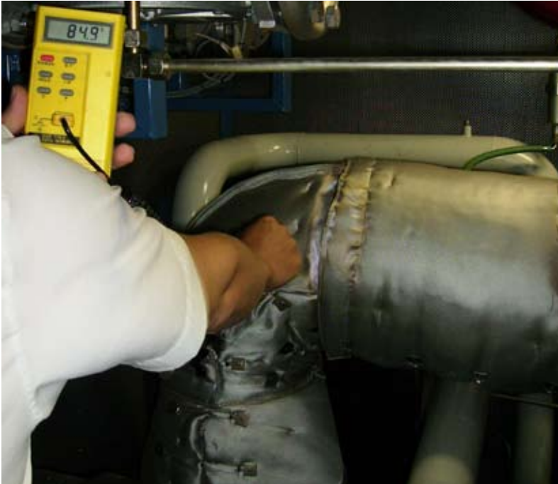
Touch temperature was reduced from 85°C (185°F) with ceramic fiber ...
